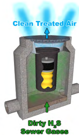
Figure 31. The Mole™ manhole insert with 20 lb. activated carbon to eliminate odors or equivalent device
