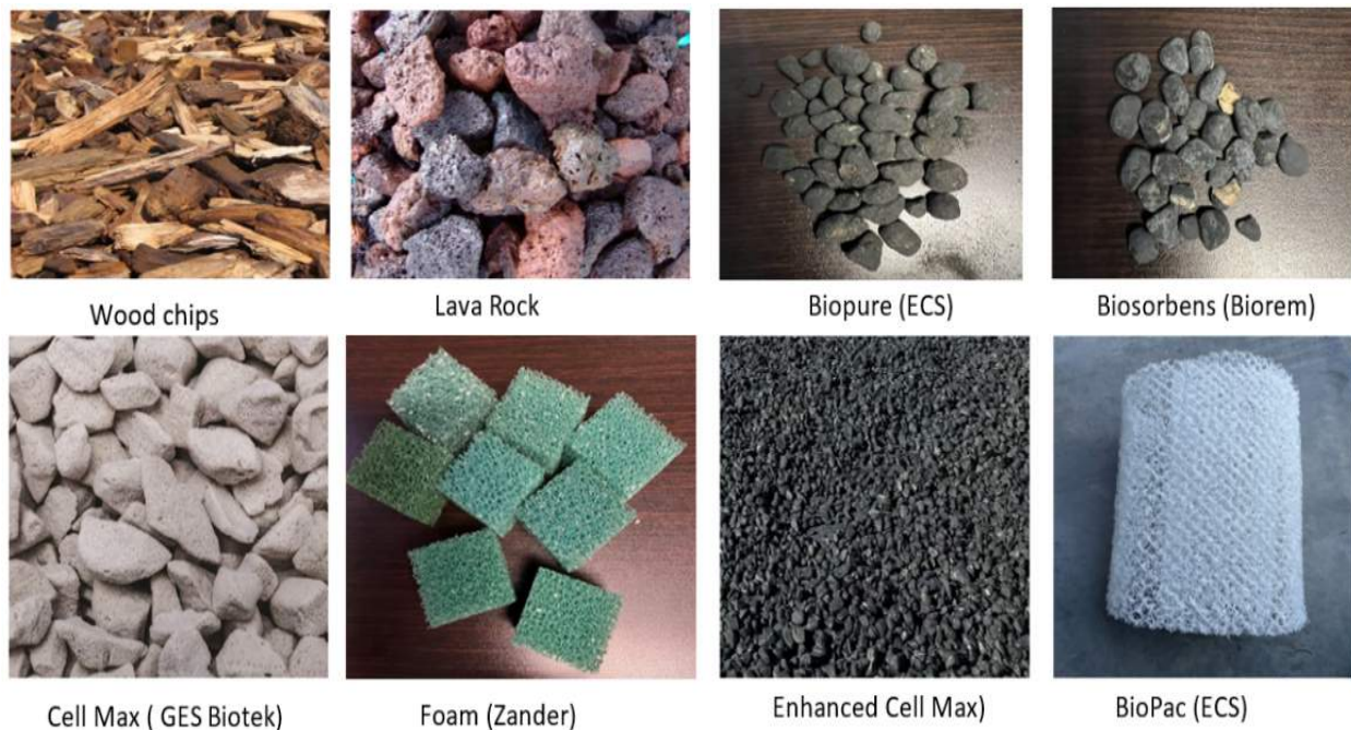
Figure 9 Typical Media Used in Bioscrubber and Biofilter Systems
