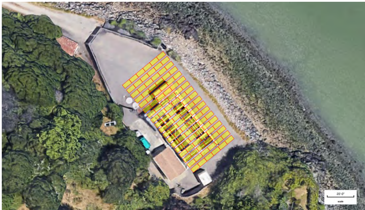
Figure 16 – Paradise Cove WWTP PV Potential
